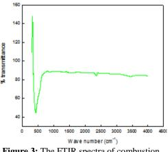
Figure 3: The FTIR spectra of combustion synthesized ZnO nanoparticles
