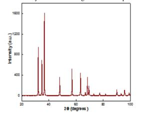
Figure 1: The powder X-ray diffraction pattern (XRD) patterns of the combustion synthesized ZnO nanoparticles
